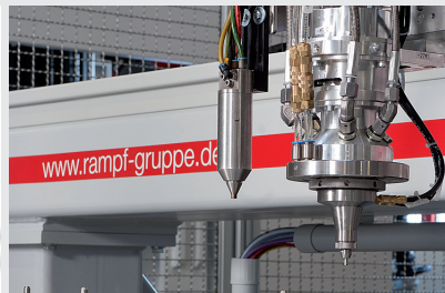
Mixing system with plasma nozzle
