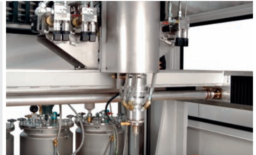
Version with 3 components and innovative mixing system MS-C
