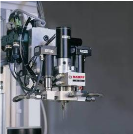
Figure 2: For dosing very small quantities, gear pumps can be mounted next to the mixing system. The pumping volume is 50 mm 3 per revolution.
